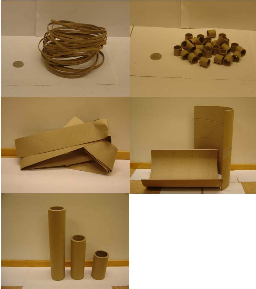
Figure 13. Photos showing the variety of paper tube waste. The paper tubes are manufactured in dimensions of 8-411 mm diameter and with varying thickness. Generally, they consist of about 10% glue (PVA or Sodium Silicate and clay), and 90% recycled paper. Figur 13. Foton som visar pappersrullar av olika dimensioner. Rullarna tillverkas i diametrar mellan 8 – 411 mm, och med varierande tjocklek. Generellt innehåller rullarna 10% lim och 90% återvunnet papper.
