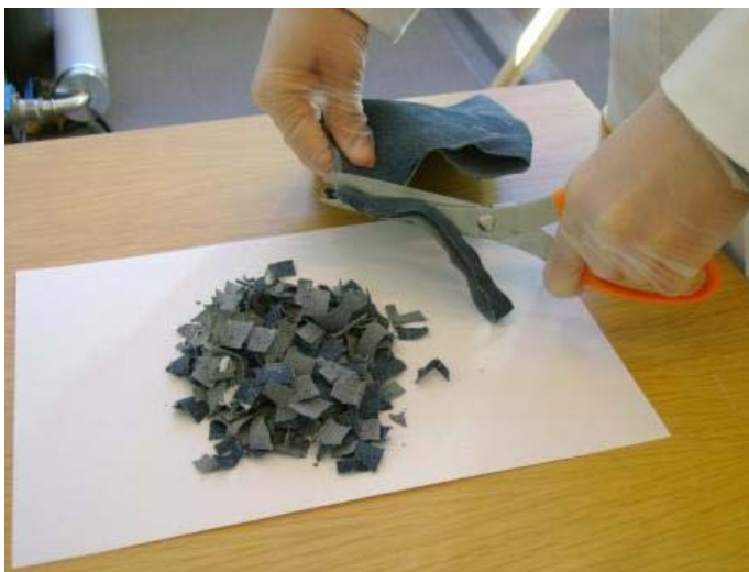
Figure 14. 1. The raw material is prepared by cutting it into small fragments. Figur 14. 1. Råvaran prepareras genom att klippas till små fragment.
