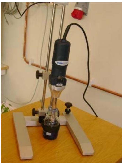
Figure 15. 2. Concentrated phosphoric acid (85 % H_3PO_4 ) is added. The mixture is homogenised every 30 min for 4 hours. Temperature is 50 °C. Figur 15. 2. Koncentrerad fosforsyra adderas och provet homogeniseras var 30:e minut under 4 timmar vid 50°C.
