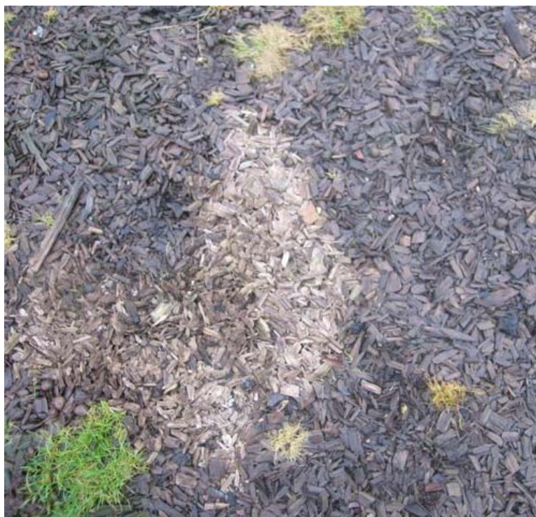
Figure 12: Picture of the biofilter's surface with two distinct zones (dried and wet)
