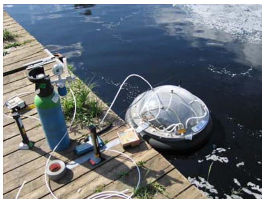
Figure 17: Picture of the sampling of the air above the leaching lake with an isolation-flux chamber
