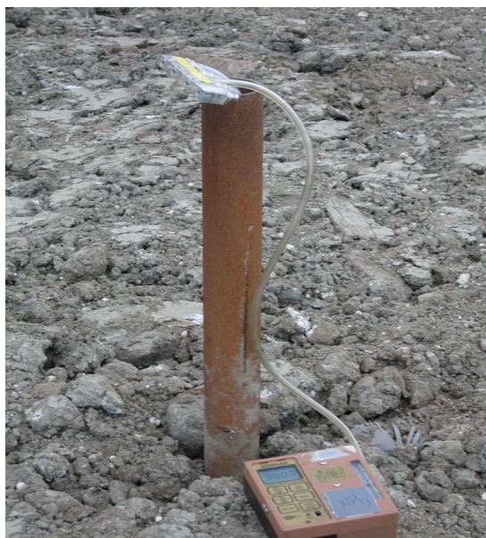
Figure 7: Picture of sampling for the gas pipe (landfill)
