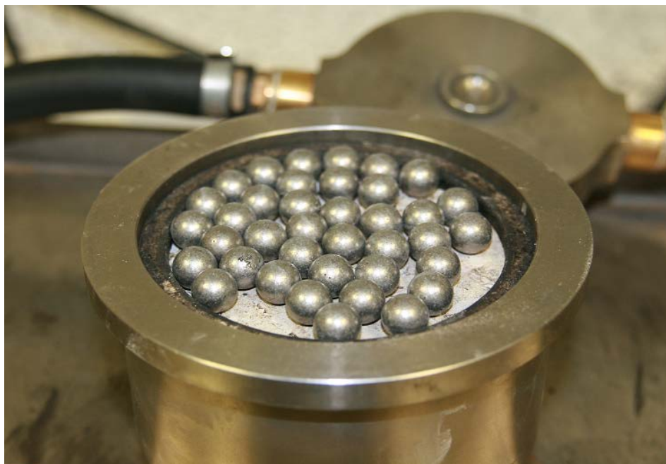
Figure 11. Abrasion test according to Prall using steel balls
