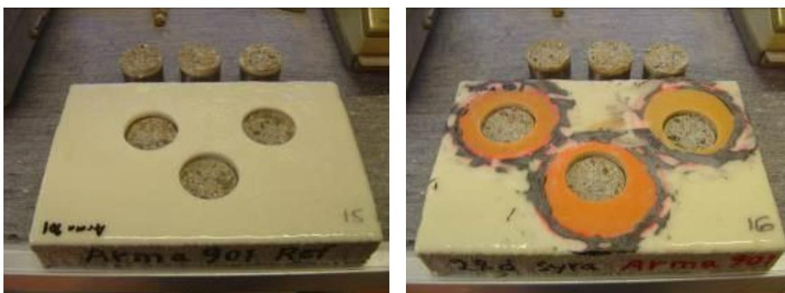
*Figure 9. Test slabs with system 8VT after pull-off testing, without exposure (left hand picture) and after exposure (right hand picture).*
