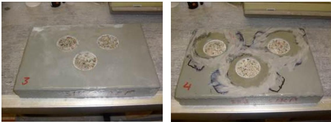
*Figure 11. Test slabs with system 11VT after pull-off testing, without exposure (left hand picture) and after exposure (right hand picture).*
