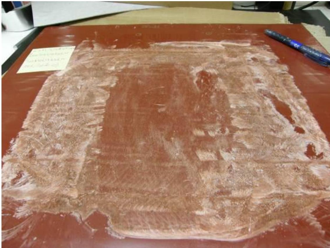
*Figure 26. Product 4G after testing according to SS EN 13892-5.*
