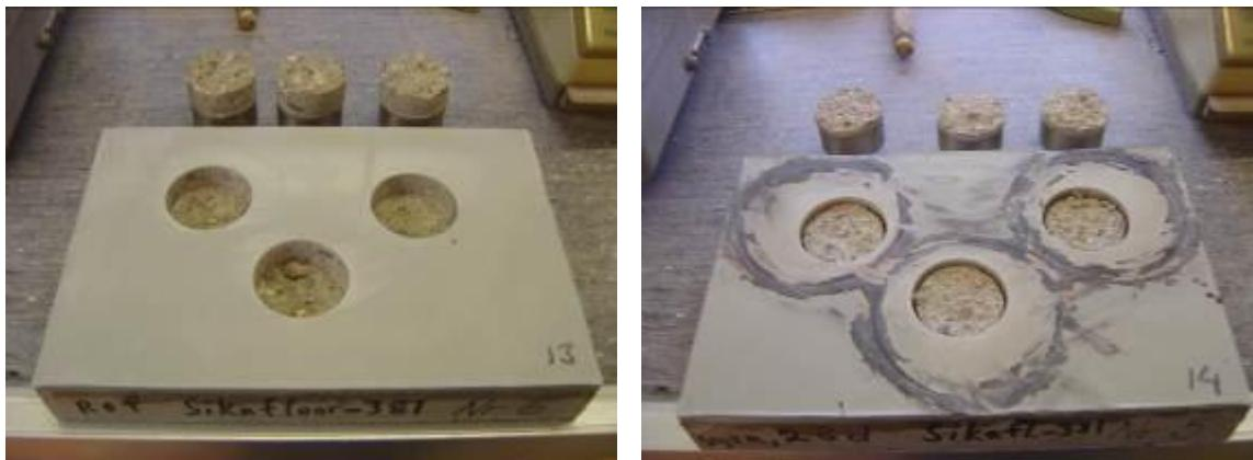
*Figure 15. Test slabs with system 6G after pull-off testing, without exposure (left hand picture) and after exposure (right hand picture).*
