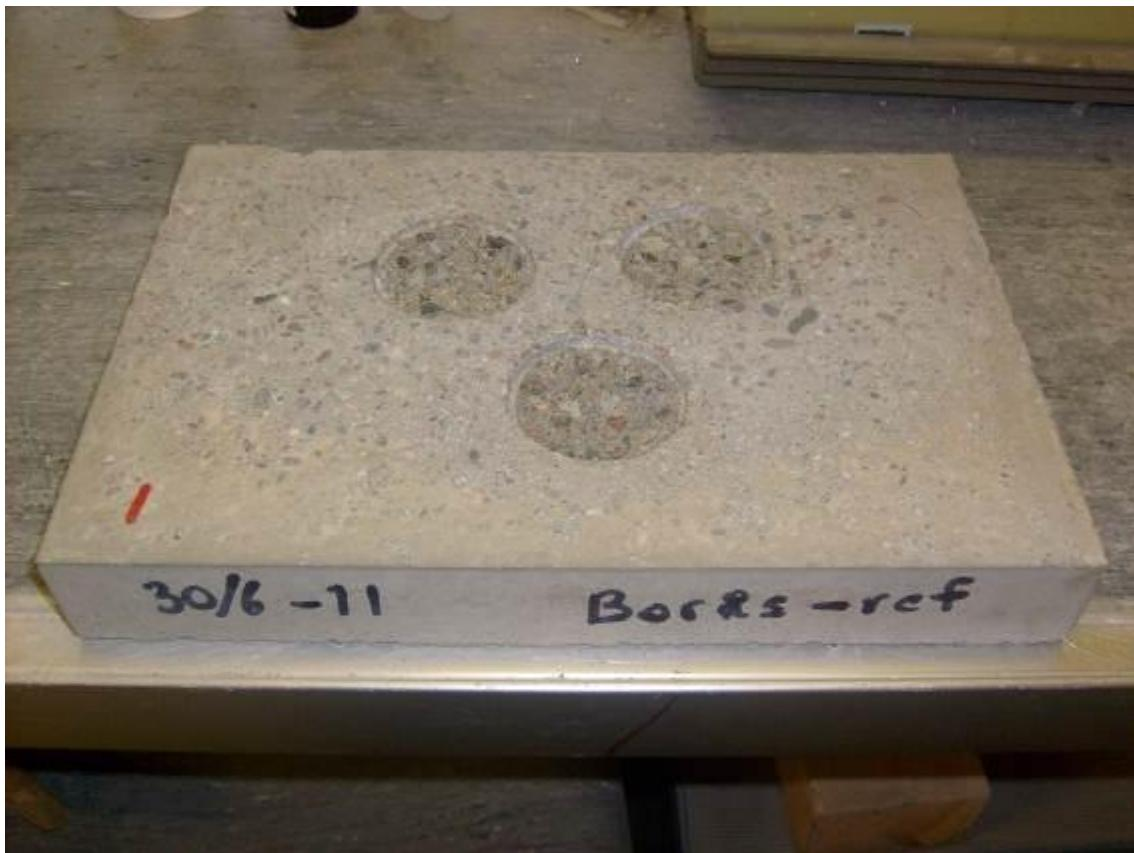
Figure 23. Reference concrete, after pull-off testing, without exposure.
