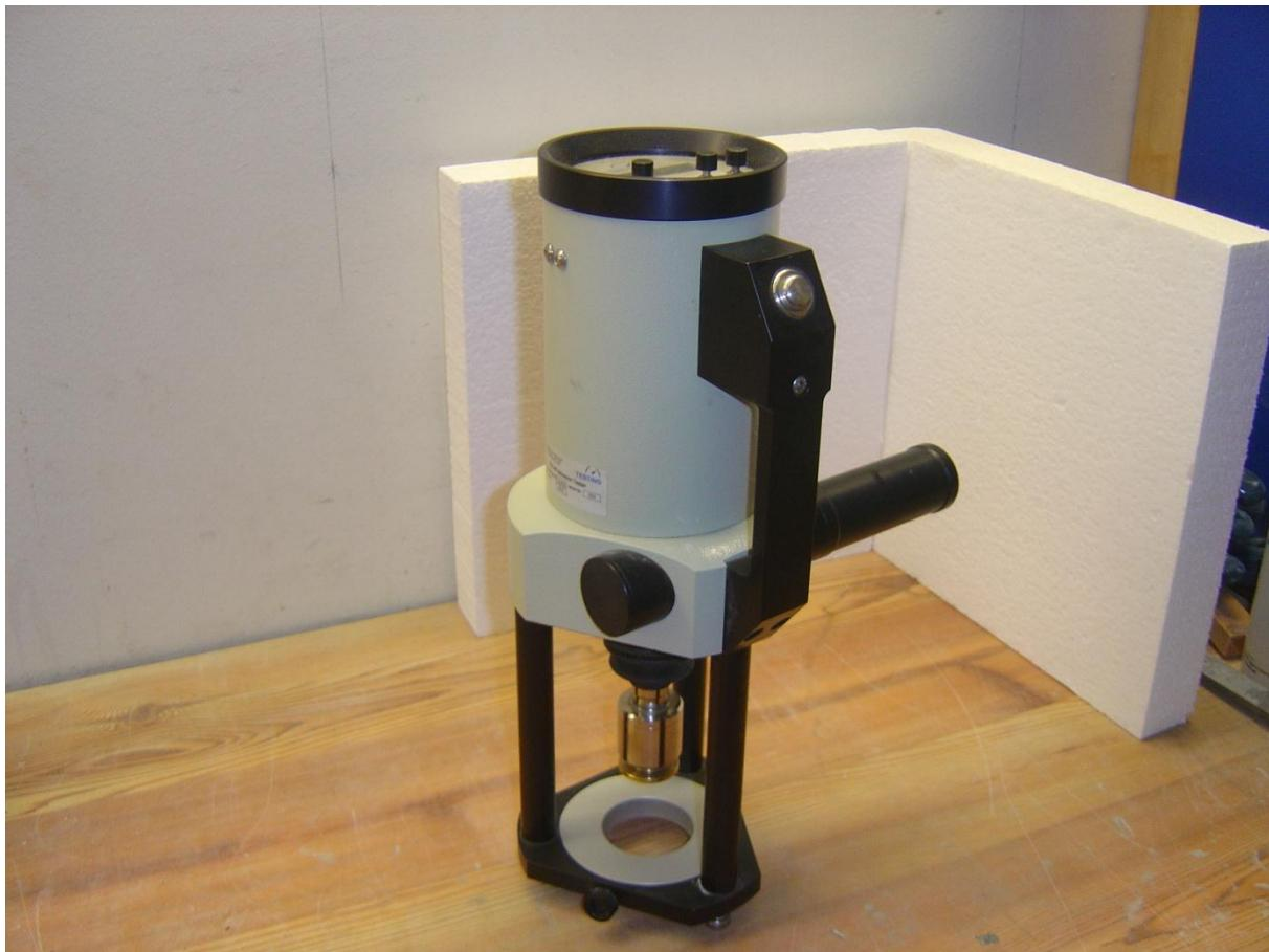
**Figure 2** Tensile bond tester for perpendicular pull-off testing.
