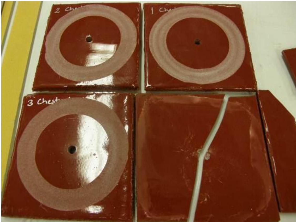
*Figure 27. Product 10VT after testing according to SS EN ISO 5470. Plus cracked sample.*
