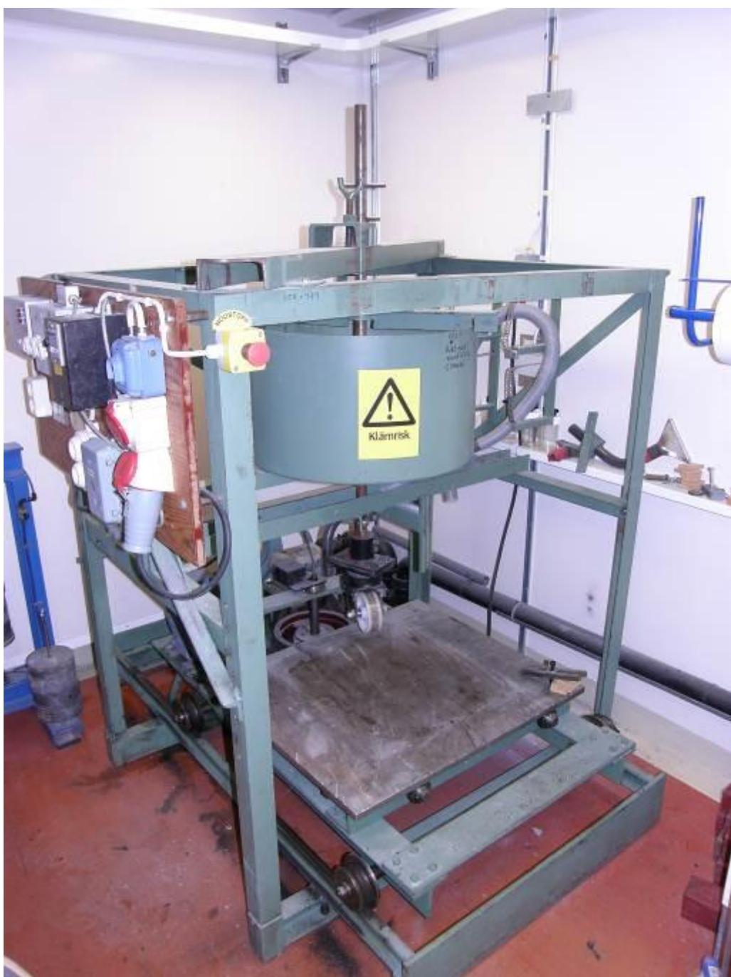
*Figure 5. Abrader equipment according to SS EN 13892-5*
