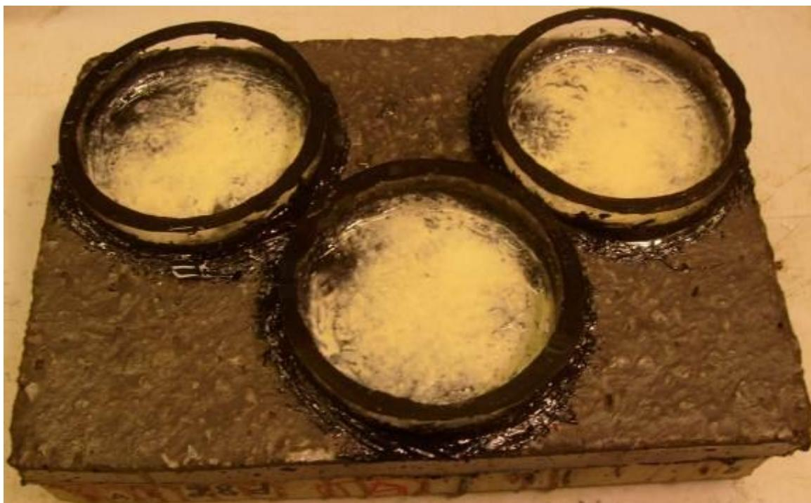
*Figure 6. Test slabs with system 1G after exposure.*
