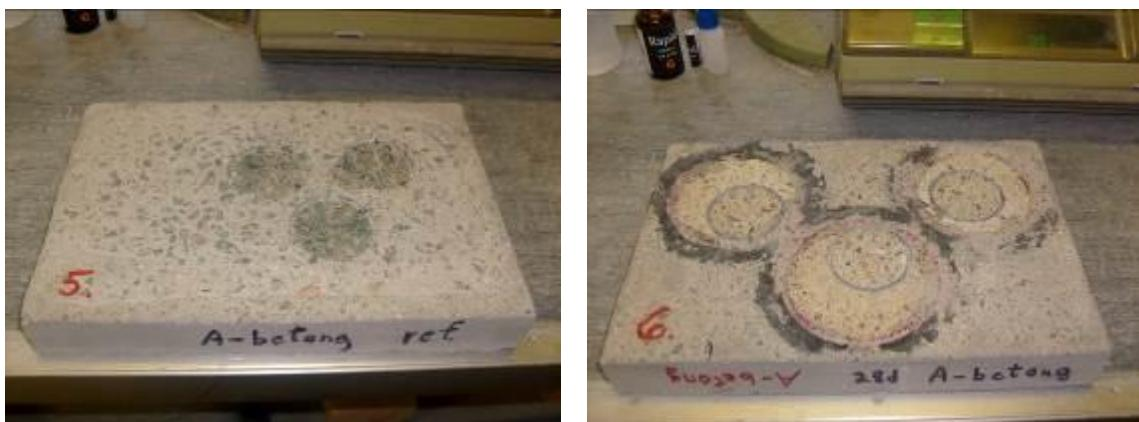
Figure 22. Test slabs of acid resistant concrete, after pull-off testing, without exposure (left hand picture) and after exposure (right hand picture).
