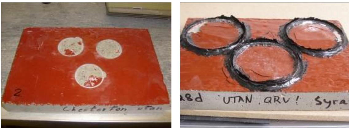
**Figure 13.** Test slabs with system 10V, after pull-off testing on non-exposed slab (left hand picture) and after exposure when pull-off testing could not be performed (right hand picture).
