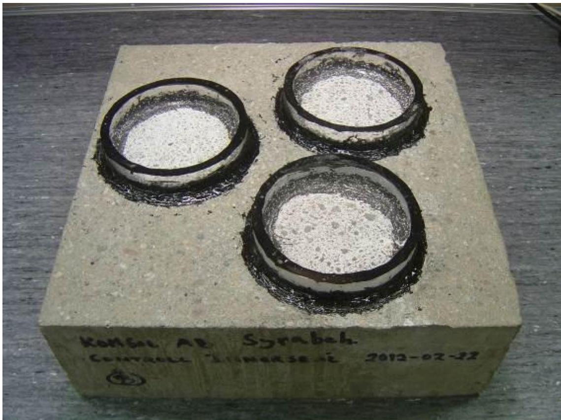
Figure 19. Silica treated test slabs, after exposure.
