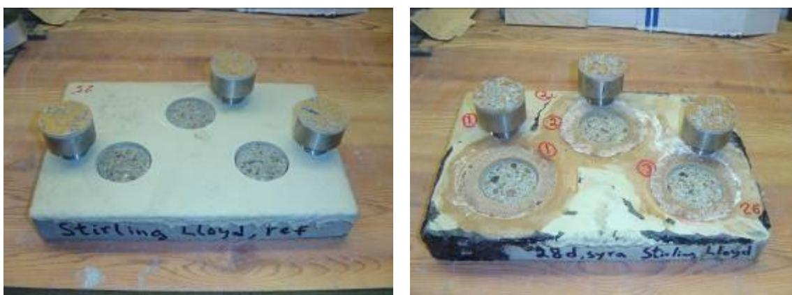
Figure 18. Test slabs with system 13VT after pull-off testing, without exposure (left hand picture) and after exposure (right hand picture).
