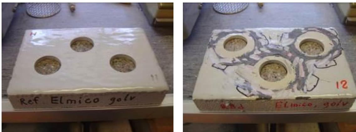
*Figure 8. Test slabs with system 3G after pull-off testing, without exposure (left hand picture) and after exposure (right hand picture).*
