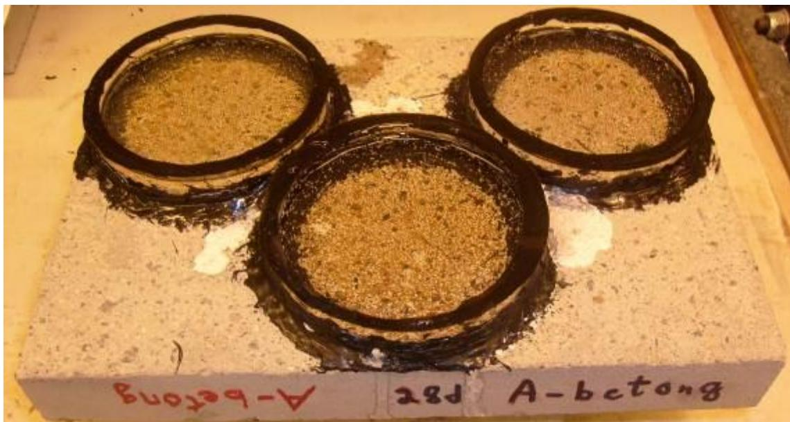
Figure 21. Test slabs of acid resistant concrete, after exposure.
