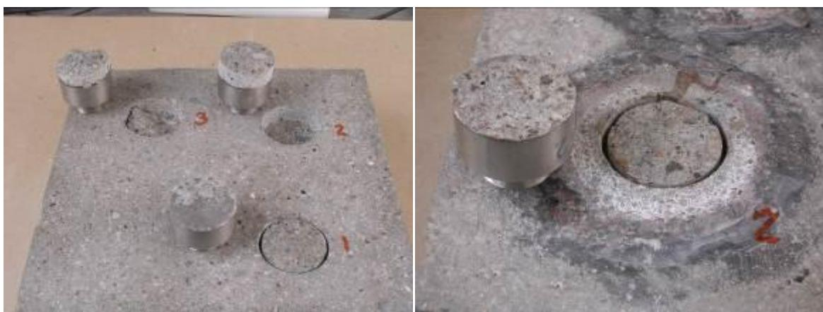
Figure 20. Silica treated test slabs, after pull-off testing, without exposure (left hand picture) and after exposure (right hand picture).
