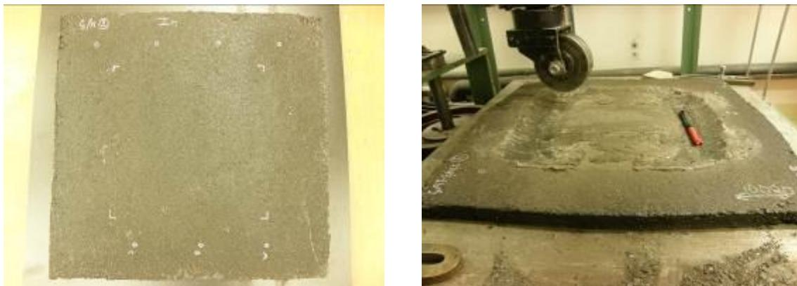
*Figure 24. Test slab of PGJA before and after abrasion testing according to SS EN 13892-5.*
