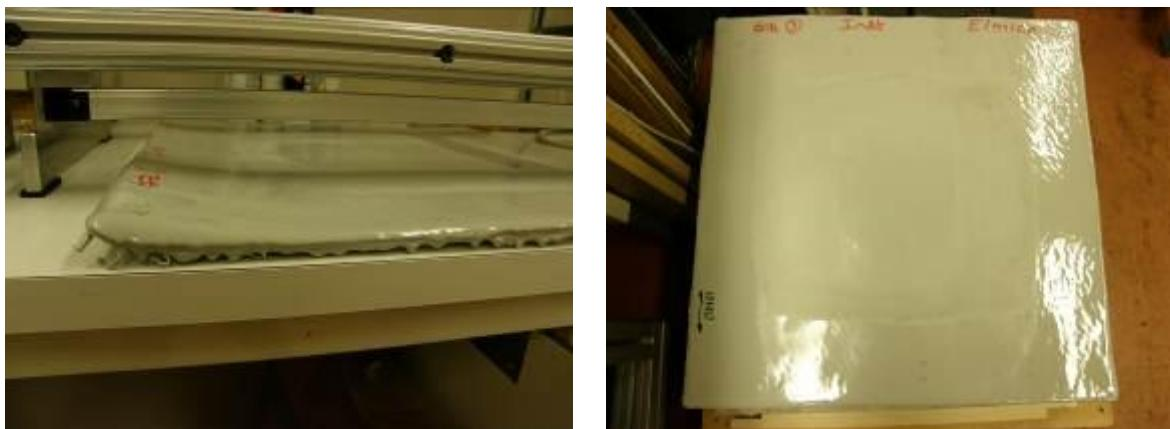
*Figure 25. Test slab of polyurea (3G), uneven edges (left hand picture) and after abrasion testing (right hand picture). Testing according to SS EN 13892-5.*
