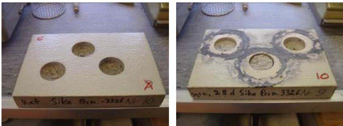
*Figure 16. Test slabs with system 12G after pull-off testing, without exposure (left hand picture) and after exposure (right hand picture).*
