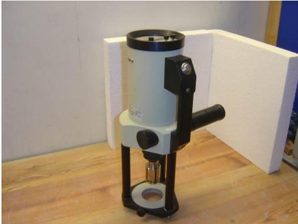
*Figure 3. Pull-off test equipment at CBI, Pull-off adhesion tester (10kN)*
