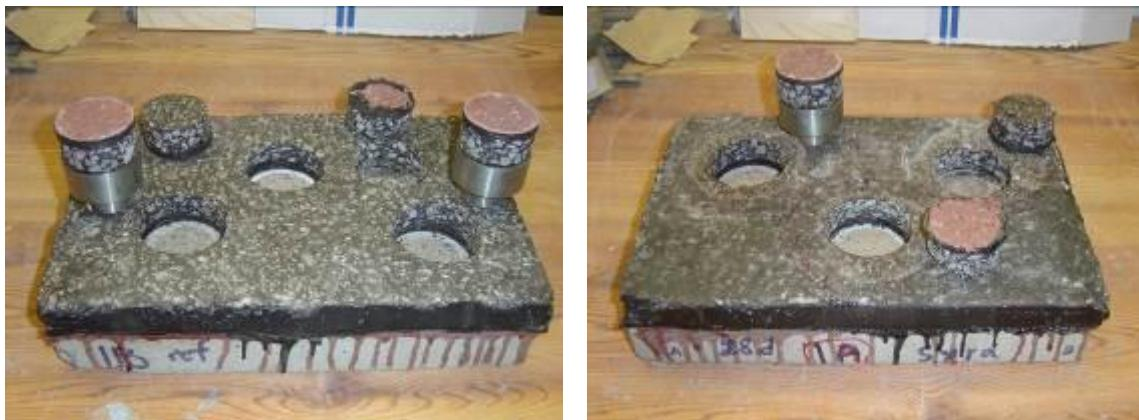
*Figure 7. Test slabs with system 1G after pull-off testing, without exposure (left hand picture) and after exposure (right hand picture) The MMA primer is pink.*
