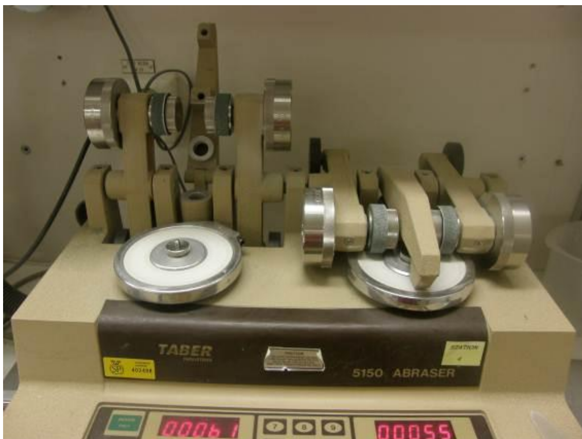
Figur 4. Taber nötningsutrustning vid SP i Borås Figure 4. Taber Abraser equipment at SP in Borås
