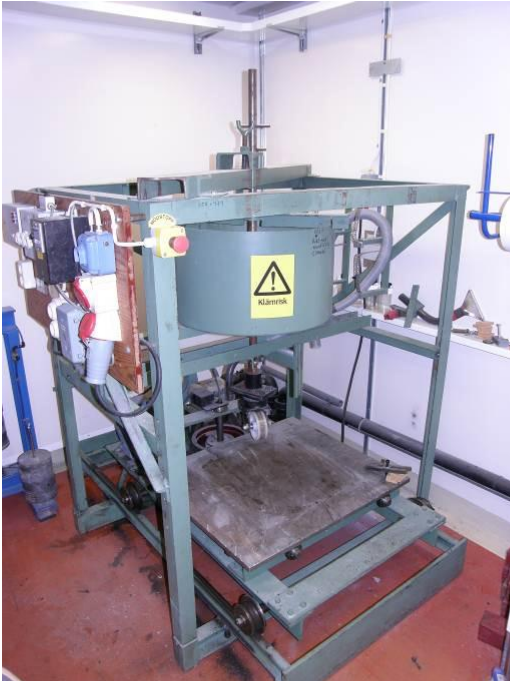
Figur 5. Slitageprovare enligt SS EN 13892-5 Figure 5. Abraser equipment according to SS EN 13892-5
